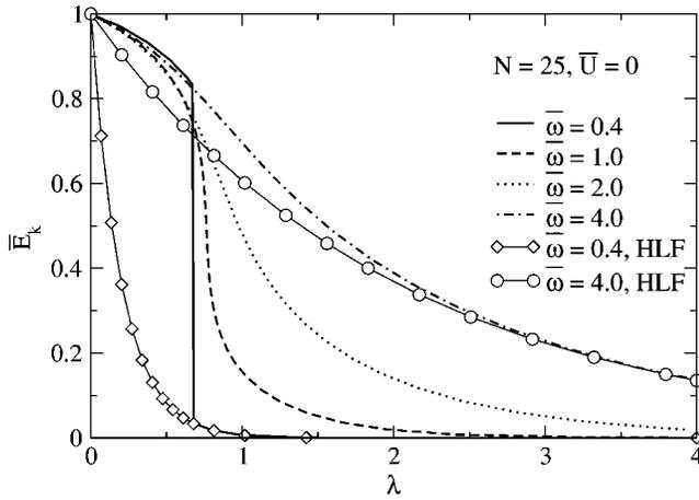
FIG. 5. Variational results for the normalized kinetic energy  $\bar{E}_k$  as a function of the el-ph coupling  $\lambda$  and for different phonon frequencies  $\bar{\omega}$ . Also shown are results of the HLF approximation (see text).
