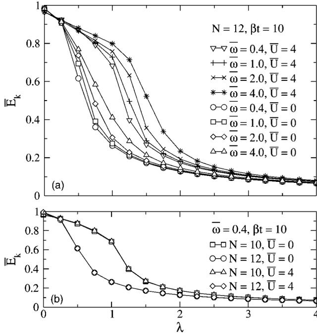
FIG. 1. (a) Normalized kinetic energy  $\bar{E}_k$  [Eq. (31)] from QMC as a function of the el-ph coupling  $\lambda$  for different values of the phonon frequency  $\bar{\omega}$  and the Hubbard repulsion  $\bar{U}$ . (b) Dependence of  $\bar{E}_k$  on the cluster size  $N$ . Here and in subsequent figures QMC results have been extrapolated to  $\Delta\tau=0$  (see text), error bars are suppressed if smaller than the symbol size, and lines are guides to the eye.
