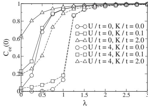
**Figure 5.** Electron–electron correlation function  $C_{ee}(0)$  as a function of electron–phonon coupling strength  $\lambda$  for a 1D system,  $\gamma = 0.1$ , and different values of the Hubbard repulsion  $U$  and the confinement strength  $K$ .
